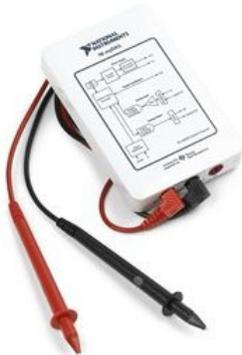
**NI myDAQ** is the powerful and portable device that students can use to measure and analyze the world around them. It is designed to work with NI LabVIEW for Education right out of the box. Start simply with built-in virtual instruments or get creative and connect your own sensors and controls.
